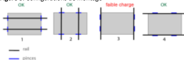
Figure 3: Configurations de montage
